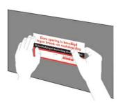
Remove part of the backing film from the back of the RPI-S Sealing sticker and place the sticker in the correct location. Rub the part of the sticker without the backing sheet firmly onto the surface.
