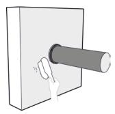
To ensure good adhesion of the RPI-S Sealing sticker, make sure the surface is clean, dry and dust-free. Do not touch the adhesive layer of the sticker while affixing it.
